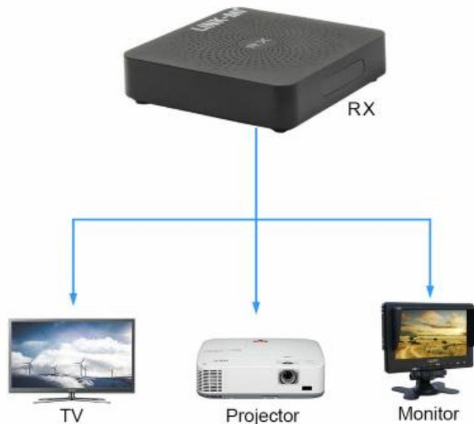
3. When the TX device RX device connected , the led on each device will be fast flashing instead of slowly flashing. The TV screen can be showing the content of the DVD when the led be flashing all the time.
